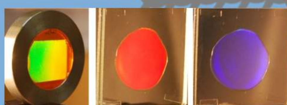
Diffraction of light by polymeric grating: Ag NP (a), LaPO4 NP (b), TiO2 NP (c) (courtesy NASU, Kiev)
