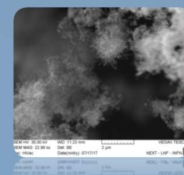
MWCNT grown on GNP (left) and epoxy nanocomposite load with 2% GNP (right)
